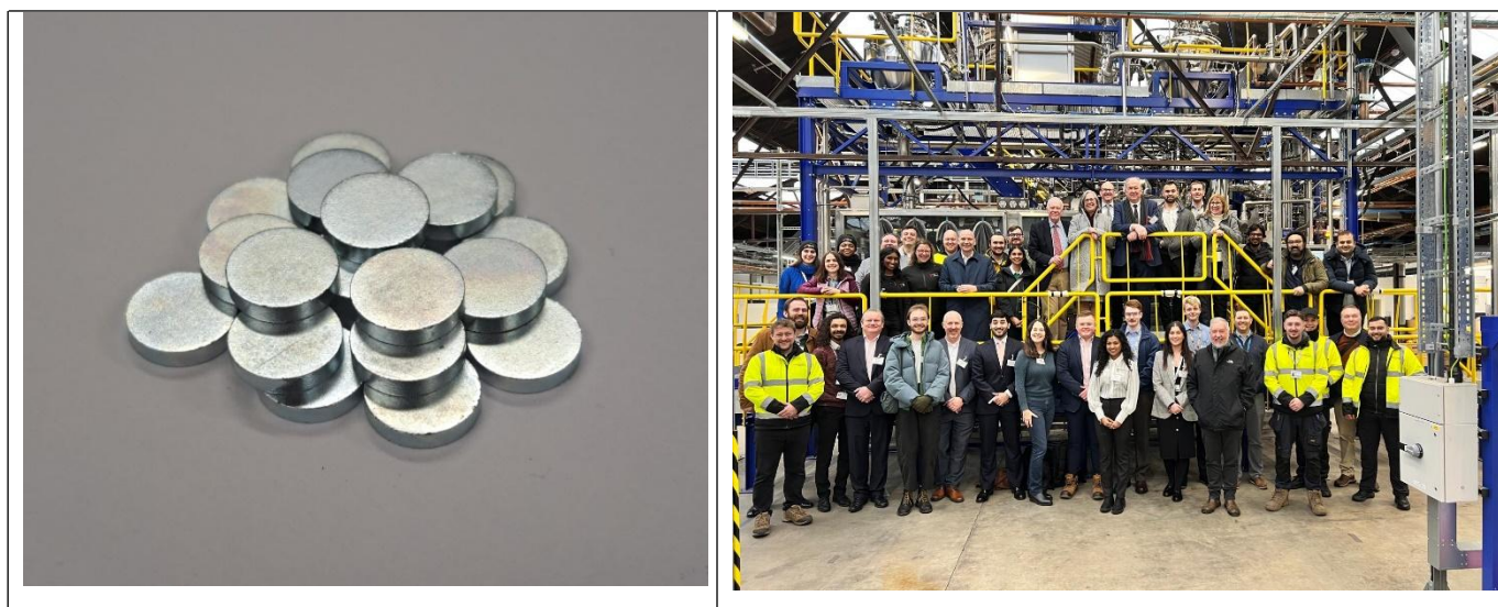
Left: Finished coated recycled NdFeB magnets for prototype demonstrations in medical devices.
