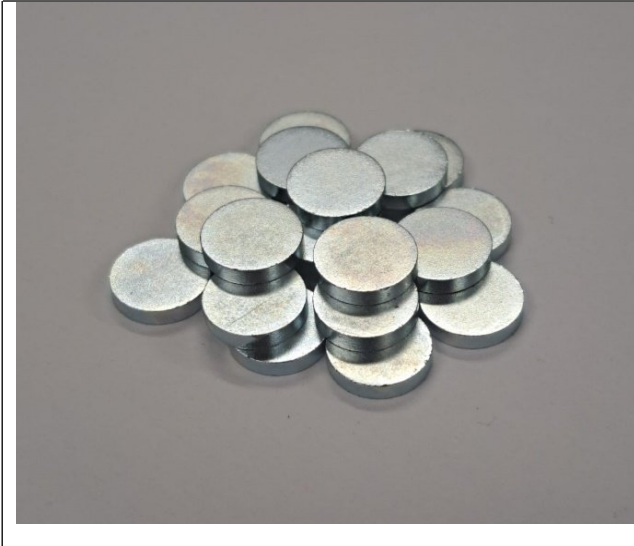
Left: Finished coated recycled NdFeB magnets for prototype demonstrations in medical devices.
