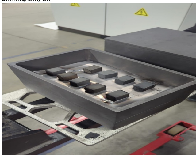
Figure 4: First magnet blocks post sintering at Tyseley Energy Park, Birmingham, UK
