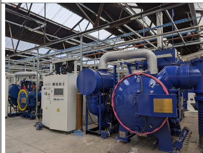
Figure 3: 50kg and 400kg sintering furnaces at Tyseley Energy Park, Birmingham, UK
