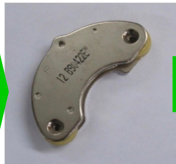
Picture B. Separated Voice Coil Assembly – NdFeB magnet inside
