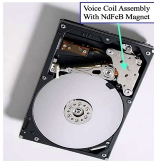
Picture A. Hard Disc drive with Voice Coil Assembly shown
