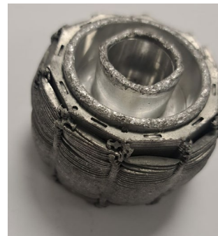
Picture B: NdFeB liberated from rotor via HPMS
