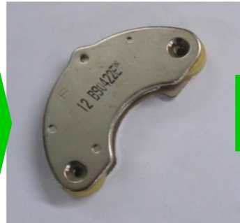
Picture B. Separated Voice Coil Assembly – NdFeB magnet inside
